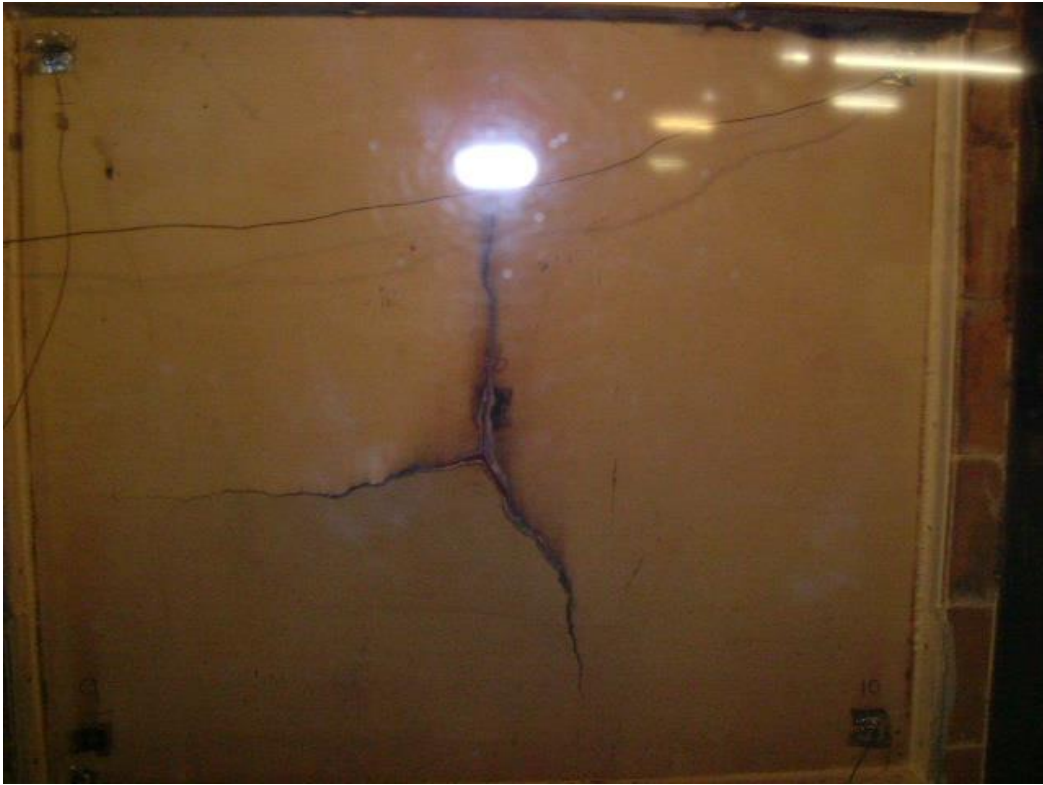
Figure 9 - Test Specimen 1 - Observation at Test Termination
