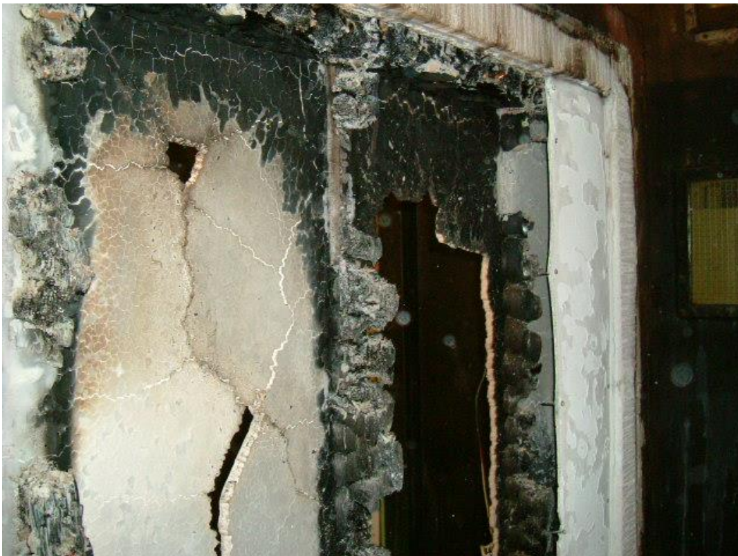
Figure 18 - Test Specimen 2 - Post Test Observation - Fire Side
