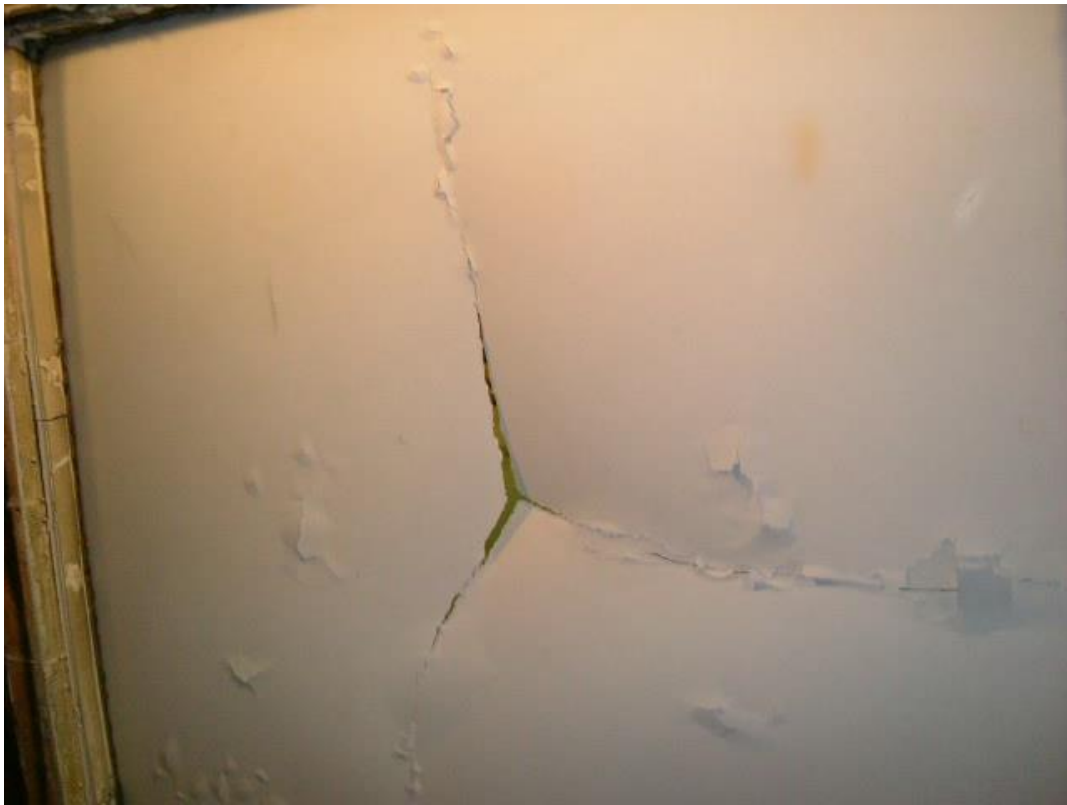
Figure 11 - Test Specimen 1 - Post Test Observation - Fire Side
