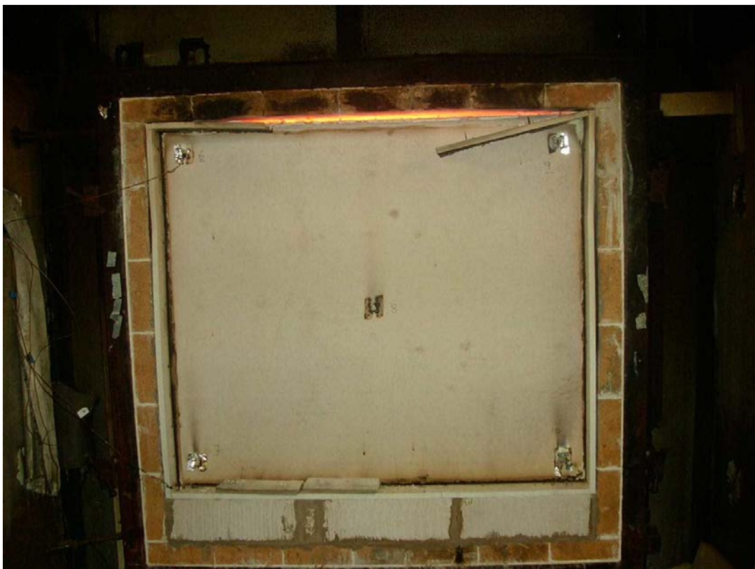
Figure 11 – Post Test Observation Fire Side Face
