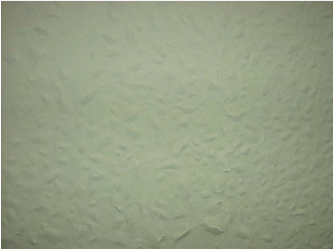
Figure 13 – Post Test Observation : Non Fire Side
